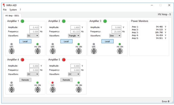
Software interface showing an HVA with 5 channels; channel 3 has the 180 V option. Channels 1, 2, and 3 in remote control with a DC offset, triangle waveform, and sine wave output respectively.
