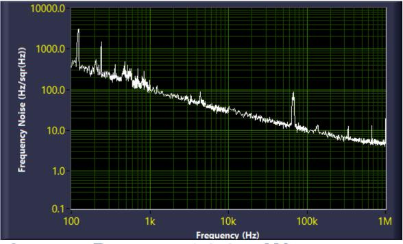
Output Power: 24.1 mW Instantaneous Linewidth: 53.9 Hz Mode Hop Free Tuning: 23.4 GHz
