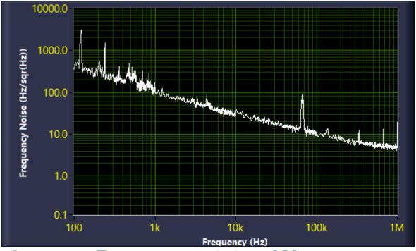
Output Power: 34.8 mW Instantaneous Linewidth: 27.8 Hz Mode Hop Free Tuning: 17.9 GHz
